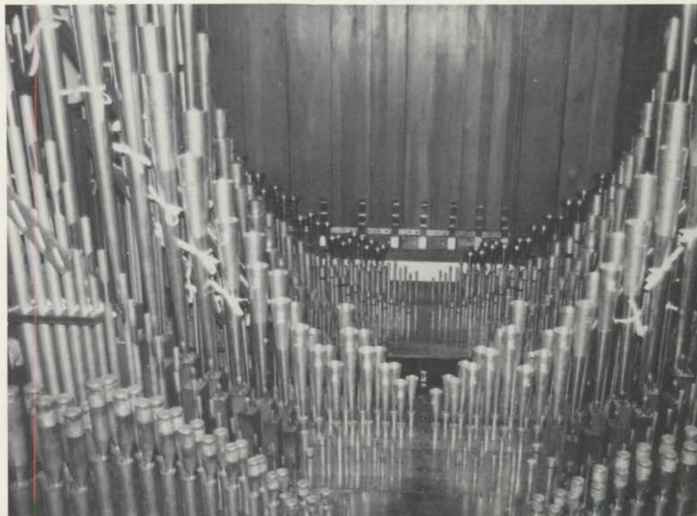
Solo: (Front to rear) Saxophone, Gamba, Quintadena, Gamba Celeste, Oboe Horn, Trumpet, Tibia, Solo String, Vox Humana. (Dan Wilke photo)
