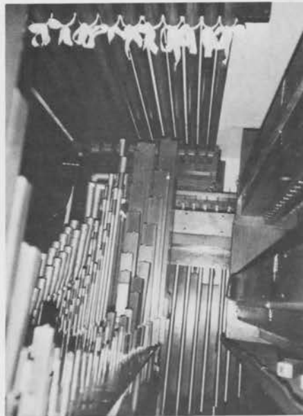
Eight-foot Salicional offset of 12 pipes, mounted on ceiling.
