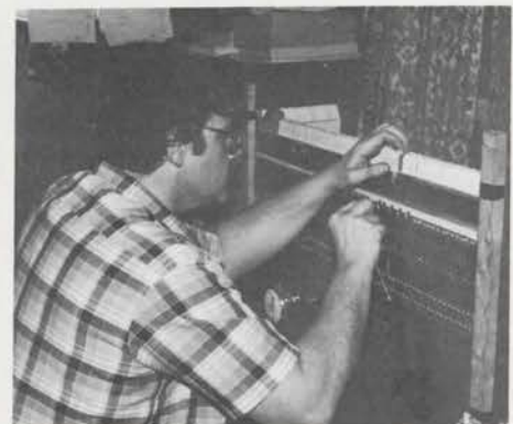
Tom Hurst installs and adjusts second touch springs on the accompaniment manual of the Redford's Barton. Bill Vogel Photo
