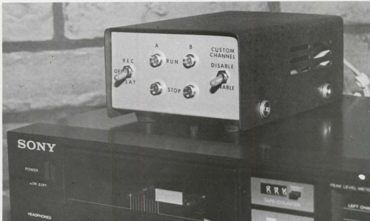
Photo 4: Typical example of the control box built for the Style E, showing the simple controls and 4 LEDs.
