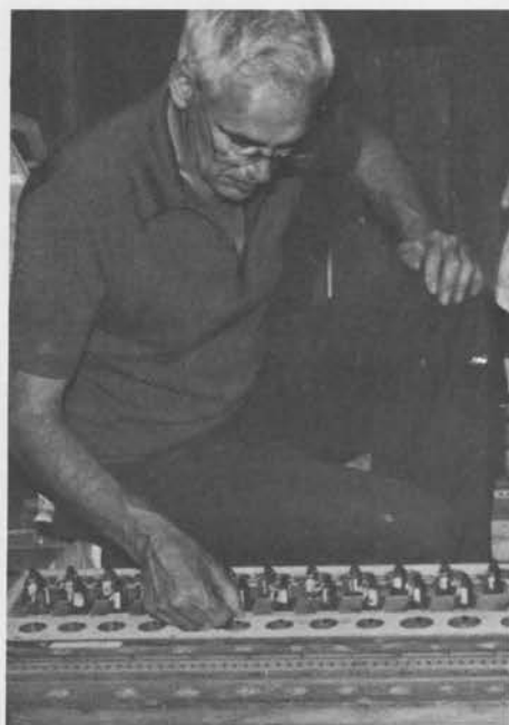
Bill Irvine checks the "puff" before sealing the chest.
