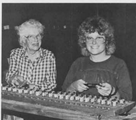
Linnea Kindig and Debbie DeCaro removing old leather and rebuilding magnets.
