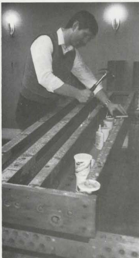
Mark Cooley driving home a dowel rod in one of several hundred holes in the main chest of the Solo division.
