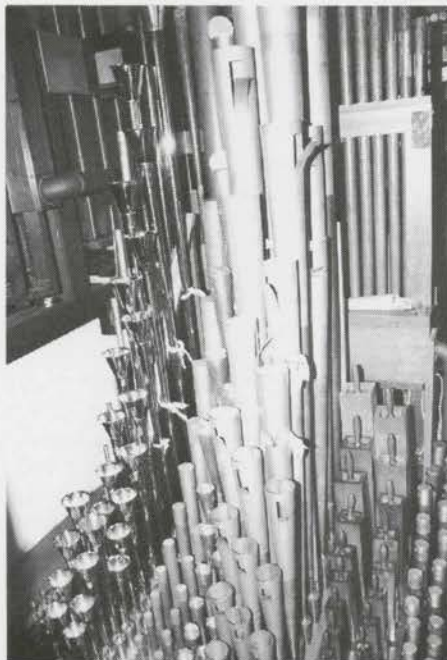
Solo chamber pipework: Kinura, Orchestral Oboe, Quintadena, Serpent, Kimball Tuba, Tibia, Vox Humana.
