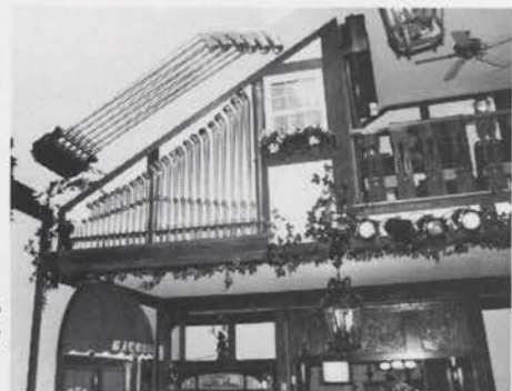
Chest bottom boards are on ribbon connectors for ease of maintenance. Dave Junchen Photo
