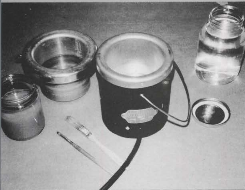
L to R: Glue jar, inner pot, brushes, one-quart glue pot, water jar.
