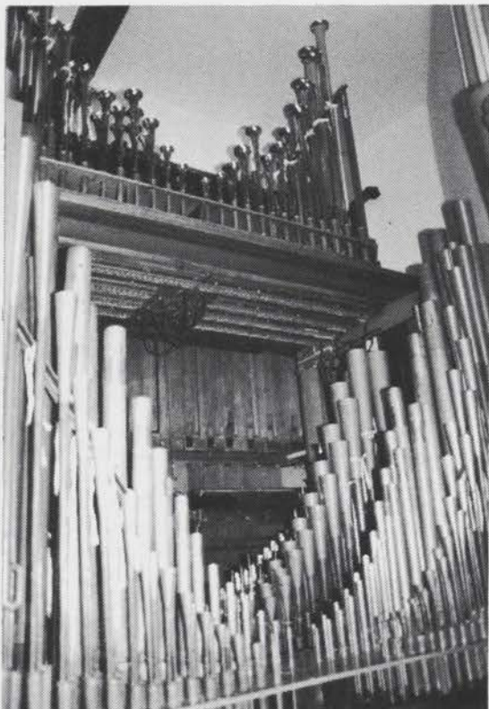
Solo chamber. The toy counter has since been erected on this side of the upper chest.
