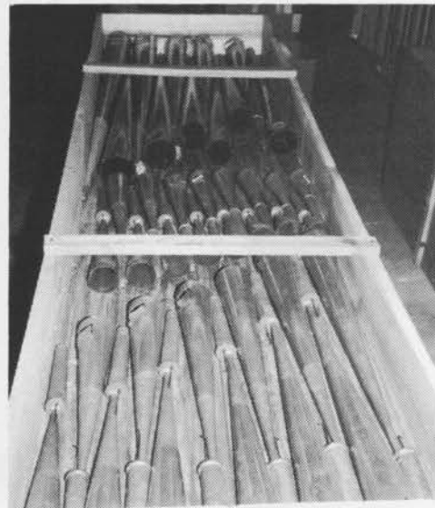
METHOD OF FITTING PIPES INTO TRAYS, WRAPPING REMOVED FOR ILLUSTRATION.
