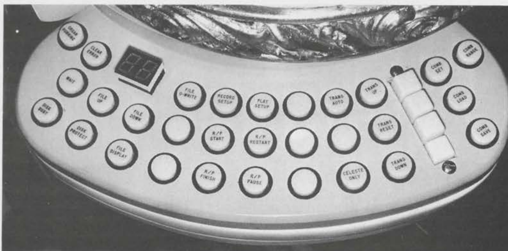
Right swingout shelf contains buttons controlling Devtonix Organ Computer Control system. The square buttons control Sostenuuto action.
