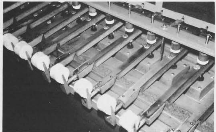
HAMMERS IN PLACE.
