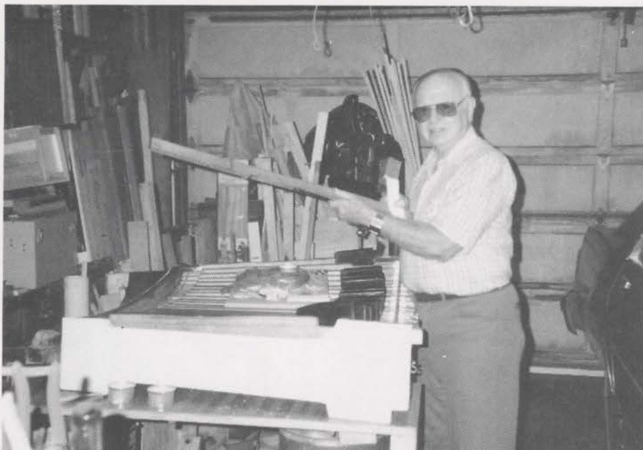
Fred Jenkins rebuilding the Fox lobby console pedal board.
