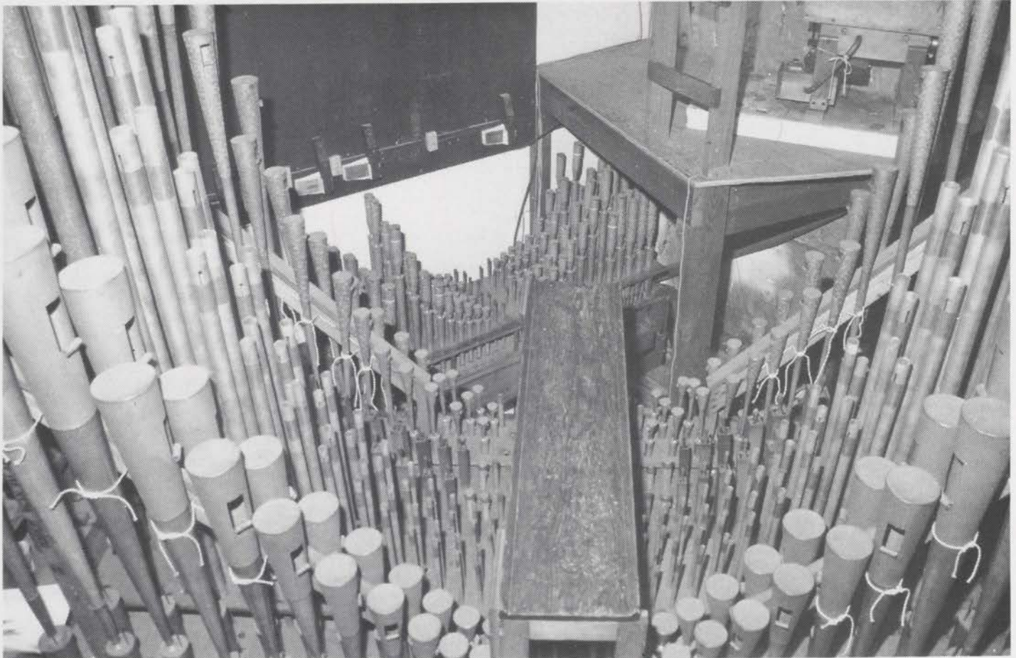
MAIN CHAMBER — lower chest showing Clarinet, Concert Flute, Diaphonic Diapason, Violin, Violin Celeste, Trumpet, Tuba.
