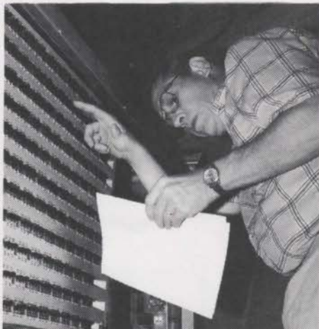
Paul Wasserman checks the setter board on the new combination action. Paul designed and engineered the electronics for the preset system.
