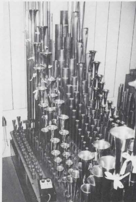
L to R: Kinura, Brass Trumpet, Orch. Oboe, Quintadena, Oboe Horn, Saxophone. Note remote "Magic Tuner" key holding device on chest.
