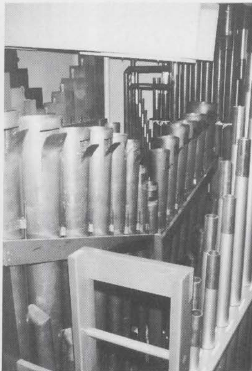
L to R: 16' Tibia (horizontal), 8' Tibia, 16' Ophicleide, 8' Spitzflute, 16' and 8' strings in background, 32' Diaphones overhead.
