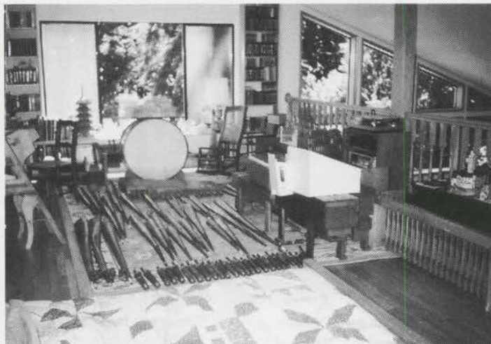
More pipes laid out on balcony prior to placing on chests. This is the Style D Trumpet. Note the many dents.
