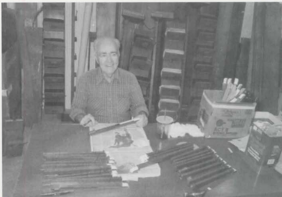
Harold Kenney refinishing the keys. Swell shade pneumatics are seen in the background. Tom Jeffery photo
