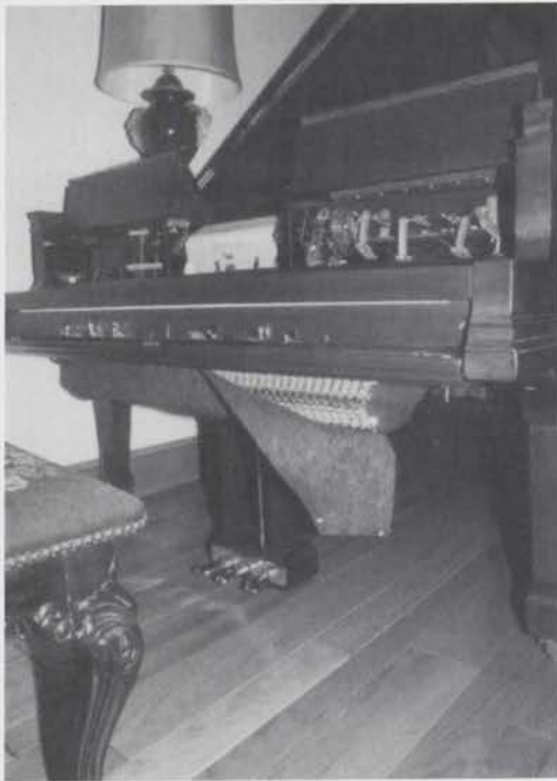
6'6" Steinway: 601 Reisner magnets below keyboard to activate pneumatics and traps.
