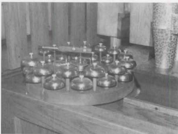
Bell Tree -- made to revolve one revolution by pressing button on key desk.
