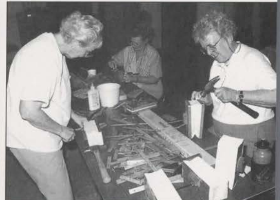
Arlene Brown, Susan Cole and Doris Ferrar releathering swell shades pneumatics.
