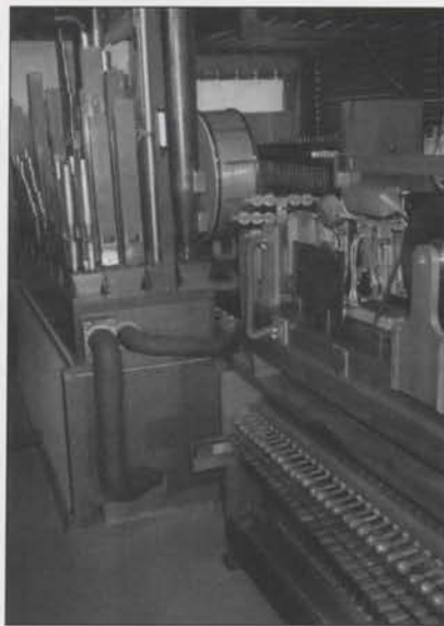
Completed installation as it appears today. Note Toy Counter is mounted on Glockenspiel at bottom, then Xylophone on top of that. Crash Cymbal not visible at end beyond the Tamborine.
