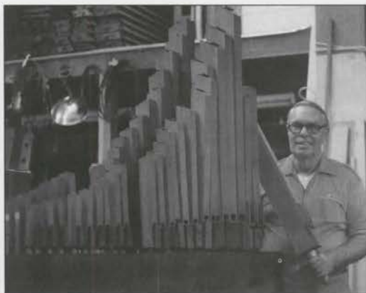
John Oien fitting new Flute Celeste on its chest for adding to Arlington Wonder Morton.
