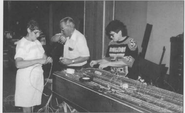
Top Left: Paul Kreglo wiring Pedal Clavier; finished console to left. Top Right: Robert Yeakle applying packing to chest bung. Bottom Left: Jack Myers and Leon Cross refurbishing 16" Tuba chest. Bottom Right: L to R: Dottie Hart, Paul Kreglo and Sue Weir wiring Accompaniment chest.
