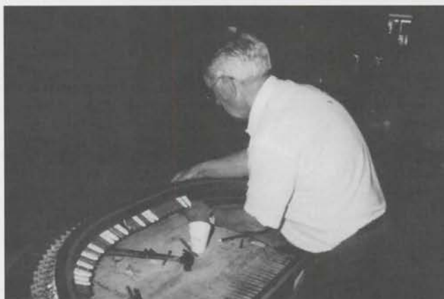
Paul Kreglo installing stop tablets in bolster.
