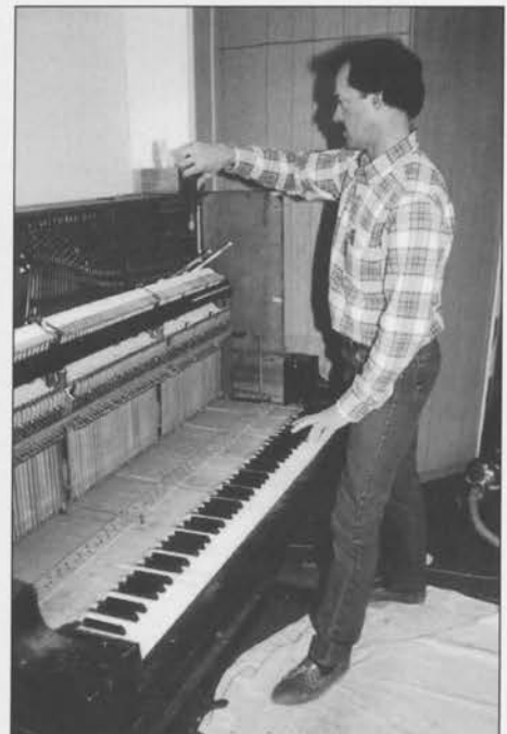
Ted Black tuning piano after installing new hammers.
