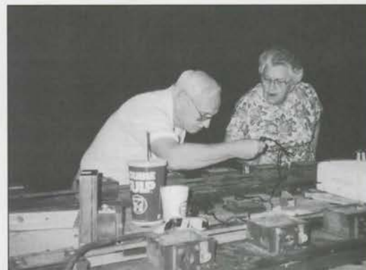
Vern and Evelyn Arthurton replacing magnets in valve boxes for Solo chamber chests.
