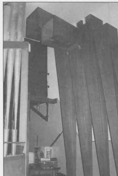
25" Wind Pressure 16' Bombarde/Tuba Mirabilis.
