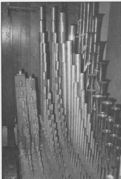
Foundation Tibia Clausa, Gamba & Celeste, Harmonic Flute, and Solo Trumpet (15" wind pressure.)
