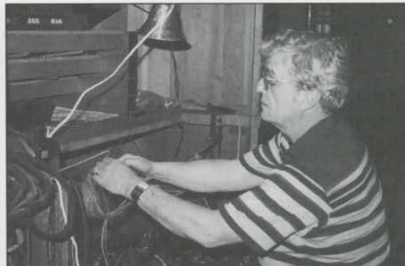
Dick Smith wires the pedal disconnect blocks. Note the general emptiness of the slave console.
