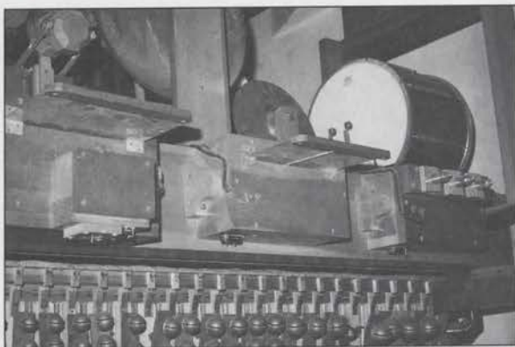
Wind & Rain Effects (aka Surf, Sand Block, and 3-Whistle Assembly) above Sleigh Bells.
