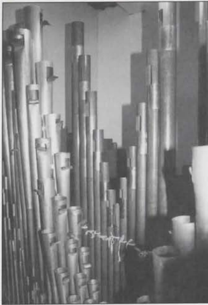
Main Chamber showing (L to R): Viol D'Orchestra, Viol Celeste, Tuba Horn, bottom octave of the 8' Dulciana.
