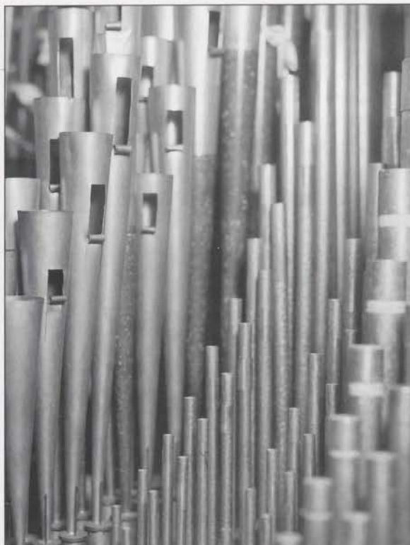
Chamber shot showing: (L to R) Tuba, 2-ranks of Violins, and Quintadena.
