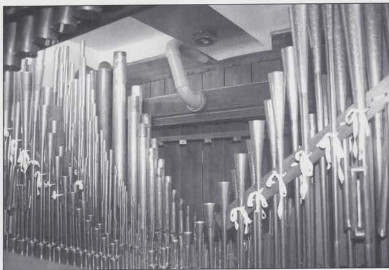
Main Chest: From Swell Shades: 1. Kinura, 2. Diapason, 3. Violin, 4. Viol Celeste, 5. Orchestral Oboe, 6. Concert Flute, 7. English Horn.
