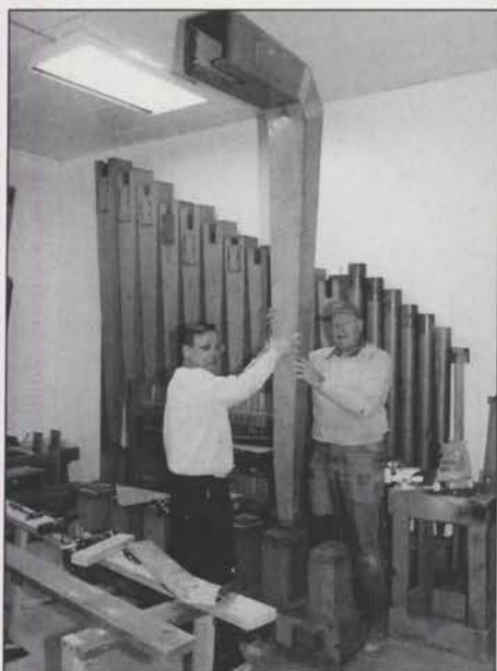
Doug Kroger at the console of Durand's 3-manual Allen digital theatre organ. At left: In Markworth's Main Chamber, Bob Markworth and Paul Kanka hoist a mitered 16' wood diaphone pipe (F#) into position -- yes, it clears the ceiling!
