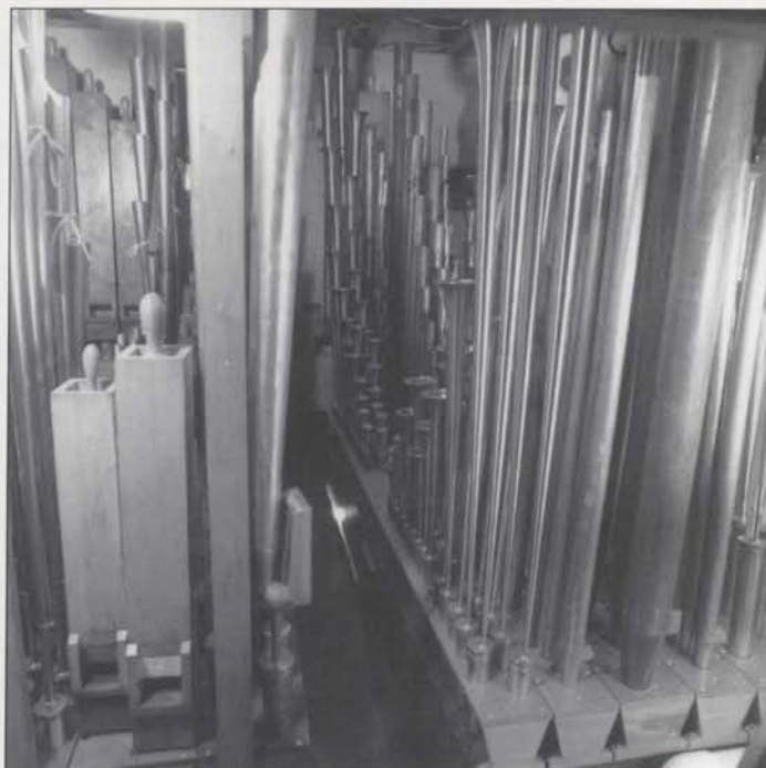
Solo Chamber. Ranks left to right: Vox Humana, Post Horn, Tibia Clausa, Tuba Horn, Brass Trumpet, String, Horn Diapason, String Celeste, Saxophone
