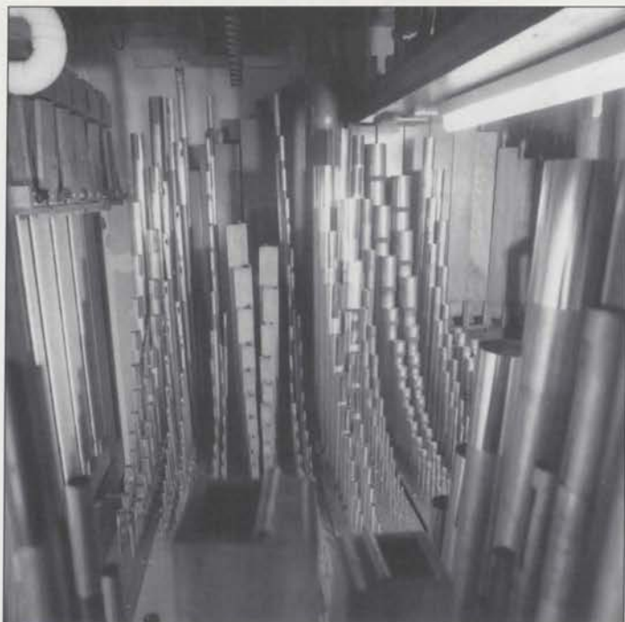
Main Chamber. Note pipes at shutter height. Ranks in order left to right: Clarinet, Orchestral Oboe, Viol d'Orchestre, Concert Flute, Viol Celeste, Open Diapason, Dulciana, Quintadena, Unda Maris, Vox Humana.
