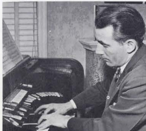
The 2 manual Page console was unusual in that it was a double bolstered factory made job for 13 ranks. The console shell was built later by Kilgen.
