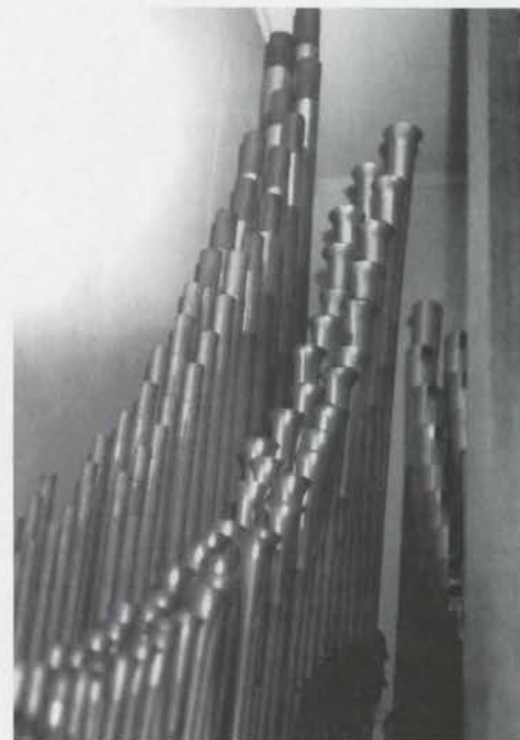
Two of the Barton's 15" w.p. ranks; Solo String (3-3/8" diameter @ cc) and Gottfried English Posthorn. Bass end of Oboe Horn can be seen right. (Solo Chamber) Scott Smith photo
