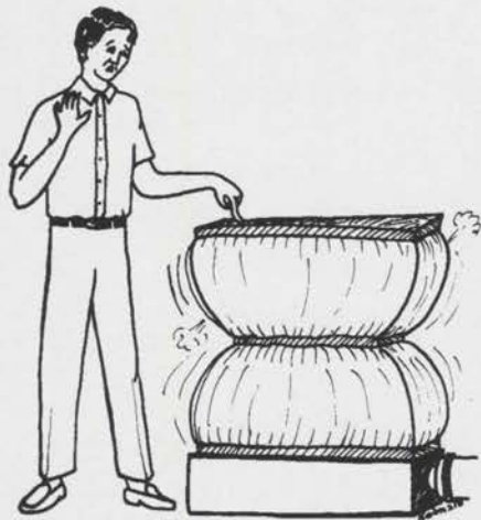
With no weights or springs to hold it down, the Regulator shot up to its full height - and static wind capacity.
