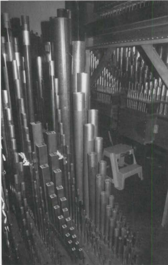
The Main chamber showing the Clarinet, Open Diapason, Violin, Flute, Violin Celeste, Gamba and Orchestral Oboe. The rear chest holds the Main Vox Humana, Lieblich Tibia, Style D Trumpet and Tuba Mirabilis.
