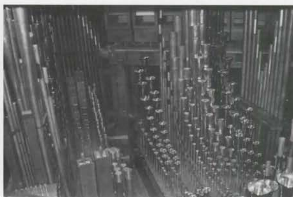
Solo Chamber: (left to right) Orchestral Oboe, Oboe Horn, Solo String, Tibia Clausa, Vox Humana, Saxophone, Solo String Celeste, Quintadena, French Horn, Trumpet. Swell shades are to left of Oboe.
