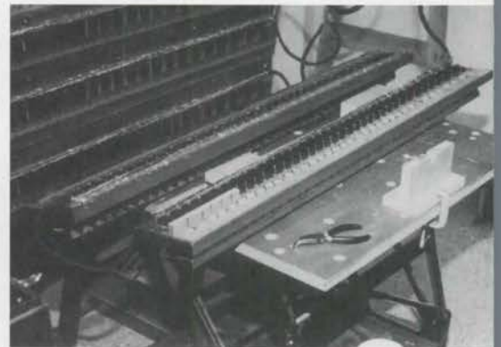
Installing new primary valves
