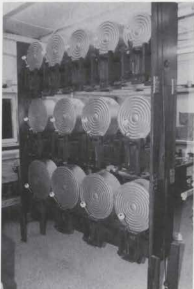
Bourdon offset chest primaries and valves
