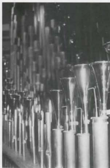
At left: 32' Diaphone back stage vibrators/resonator bases.
