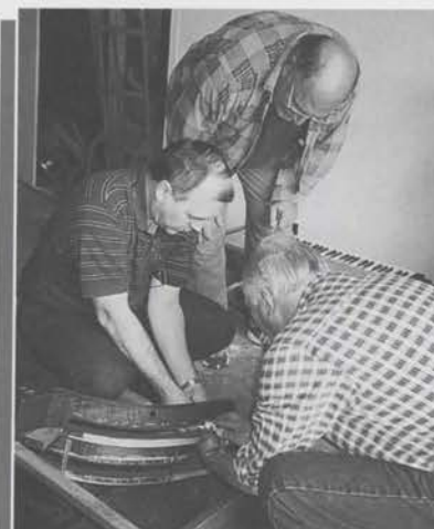
Rick Mathews, top, helps Bob Acker and Don Peterson check spacing and mounting for new stop rail.
