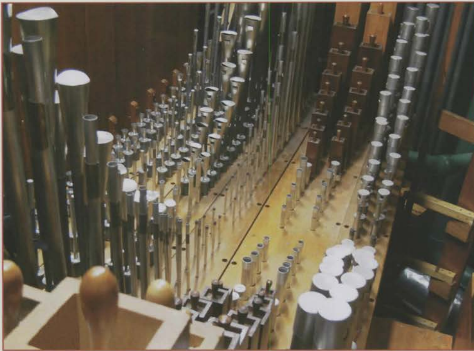
EL CAP PIPES: Peering through the Brass Sax, across the Vox Humana, the Murray Harris redwood Tibia pipes are immediately recognizable amidst a sea of Wurlitzer pipework. The pipes were re-scaled (up) one note for a subtle increase in weight and volume.
