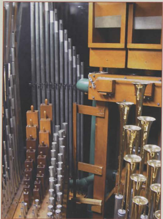
TIBIA, VOX and SAX: The often-heard combination of Tibia, Vox and Sax are visually depicted here, including the enormous 16' Tibia offset in the upper right hand corner.
