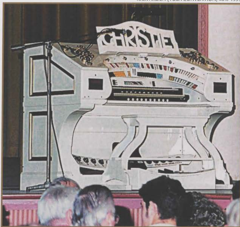
Two-Manual console ex Lyceum Theatre Sydney controls the Blakett & Howden pipe organ.
