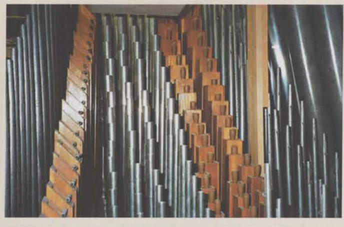
Part of Swell main chest with, from left, Dolce Celeste, Open Flute, Salicional, Voix Celeste, Stopped Flute, Dolce Flute
