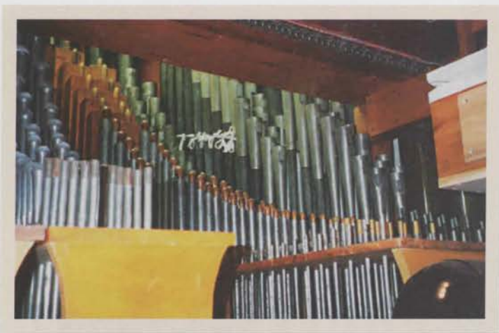
Lower level Foundation Chamber, from left, Orch. Saxophone, Lieblich Flute, Diapason and Tuba
