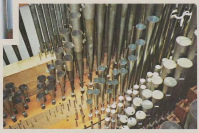
Looking down on Main Chamber, front to back, Ophicleide, M. Tibia, Oboe Horn, Vox Humana, Post Horn, Viol d'Orchestra, Tuba Horn, VDO Celeste, Quintadena, and Krumet.
