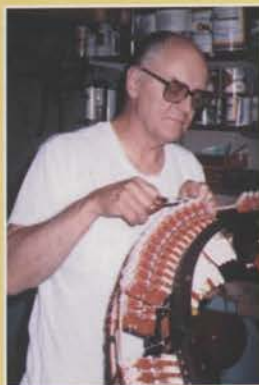
Matrix wiring of double row stop rail.
