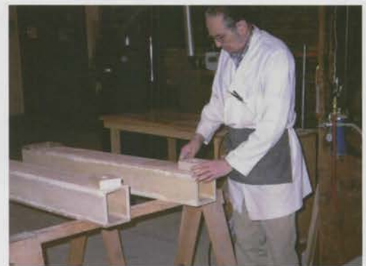
Wood pipe construction in Artisan pipe shop.
