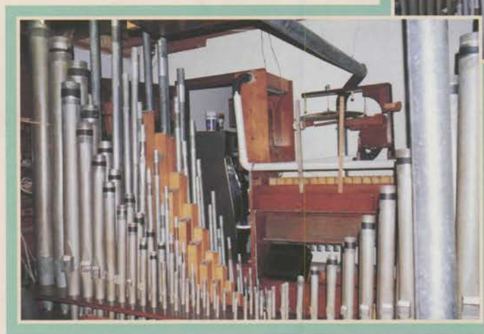
Main chest—Diapason, Phonon, VDO Celeste, Concert Flute, VDO, Deagon harp and crash cymbal.
