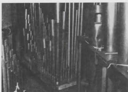
FOUNDATION CHAMBER (L to R): Möller 8' Open Diapason extension, Kimball Tuba, Kimball, Viol Celeste and Skinner, Gross Gamba. Tuba extension right foreground.
