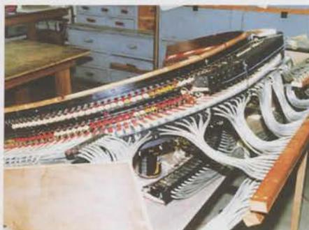
At Ken's shop the lower and upper stop rails are being reassembled.
