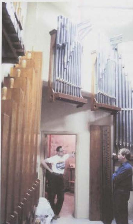
Offsets were placed high in the 15 foot tall chambers to help the sound get out. (Note door at lower middle.)
