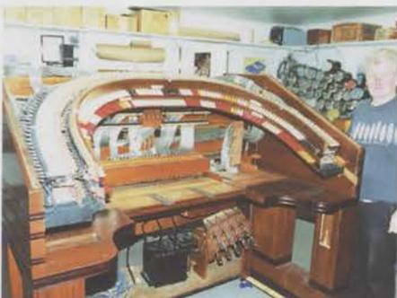
The console shell is being loaded with sub assemblies. The black object at the bottom is the original 250 stage crescendo switch with cancel pneumatic.
