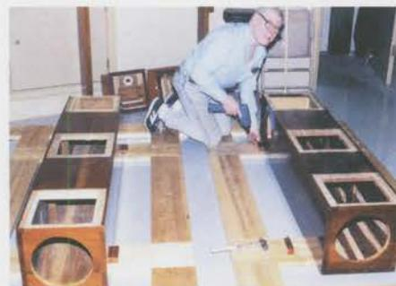
*Chamber assembly starts from the floor up with reservoir trunks mounted on new ground frames.*
