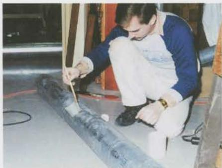
*The Berkeley organ receives its most important set of pipes, the soldered steel wind line.*
