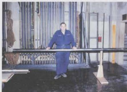
*Pipes were straightened, undented and rounded using various diameters of mandrels mounted upstage right.*
