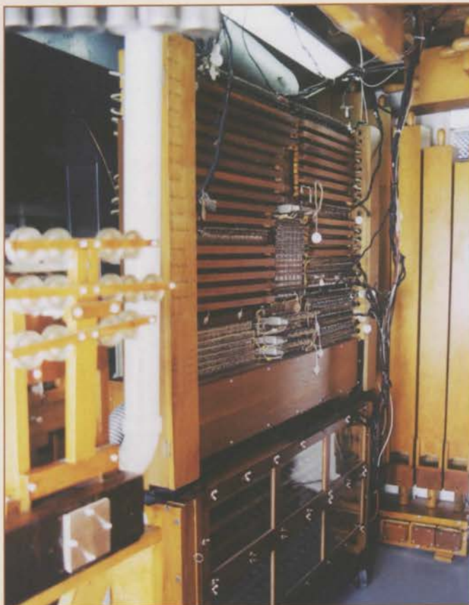
Above: View of 9 rank main chest from opposite of the swell shades. Starting in front: Vox, Oboe Horn, Open Diapason, Salicional, Flute, Viox Celeste, Tibia (hidden from view), Clarinet, Orchestral Oboe.
