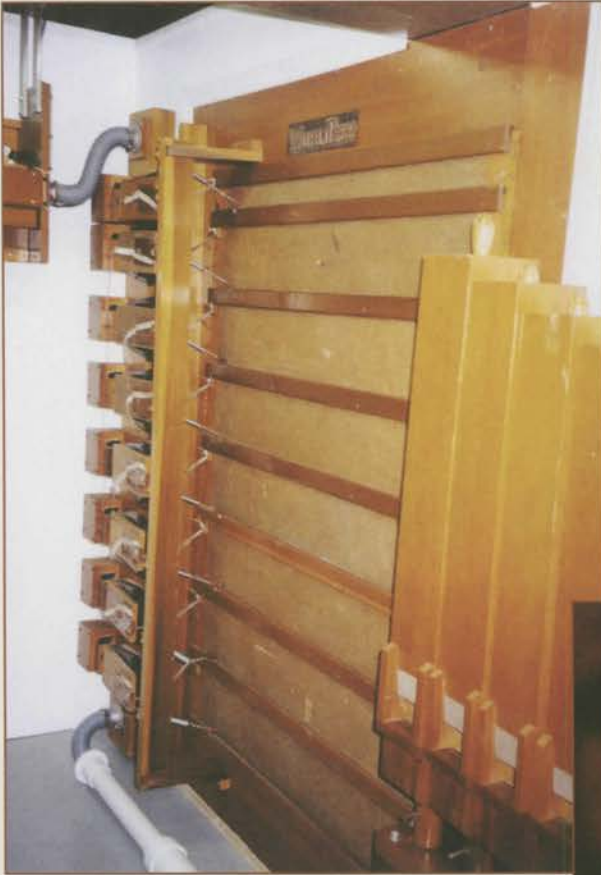
Wurlitzer 8 blade studio style Swell Shades. Tibia Offset Chest on the right.
