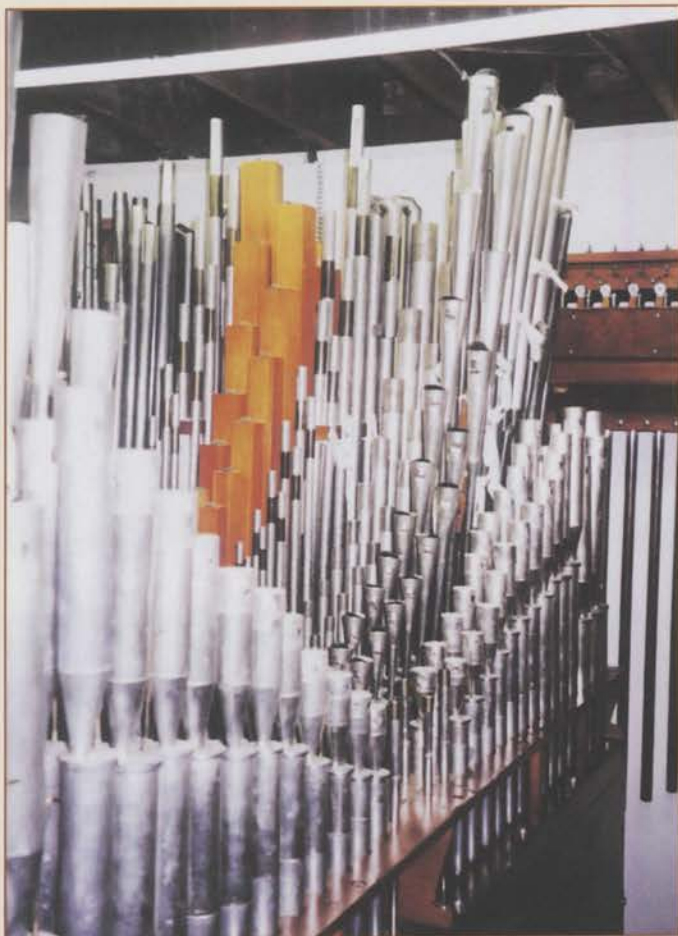
Above: View of 9 rank main chest from opposite of the swell shades. Starting in front: Vox, Oboe Horn, Open Diapason, Salicional, Flute, Viox Celeste, Tibia (hidden from view), Clarinet, Orchestral Oboe.
