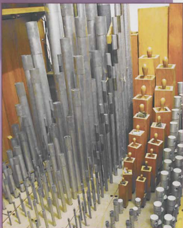
Foundation Chamber—(L to R) Open Diapason, Gamba, Harmonic Flute, Gamba Celeste, Tibia Clausa, Vox Humana.
