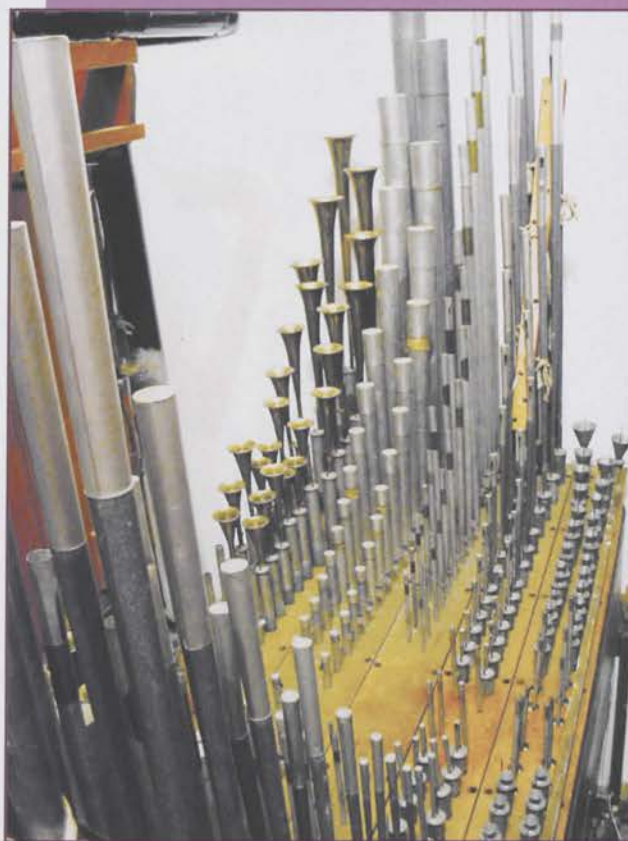
Orchestral Chamber Second Chest—(L to R) Brass Saxophone, Quintadena, Solo String, Orchestral Oboe, Kinura.
