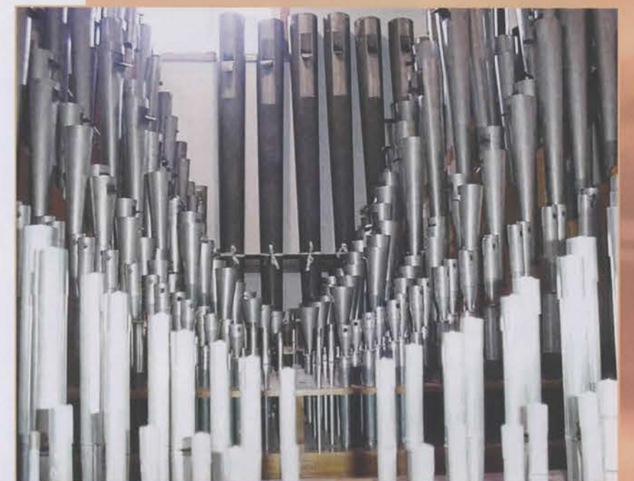
Organ Chamber—Partial Open Diapason, Vox Humana, Tibia, Style-D Trumpet, Tuba Horn, English Post Horn. Rear wall: 16' Trumpet Extension.
