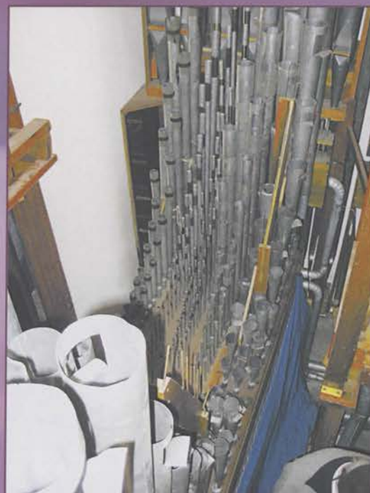
Main Chamber Chest Two—(L to R) Clarinet, Viol and VDO Celeste, Salicional, Horn Diapason, Style-D Trumpet.
