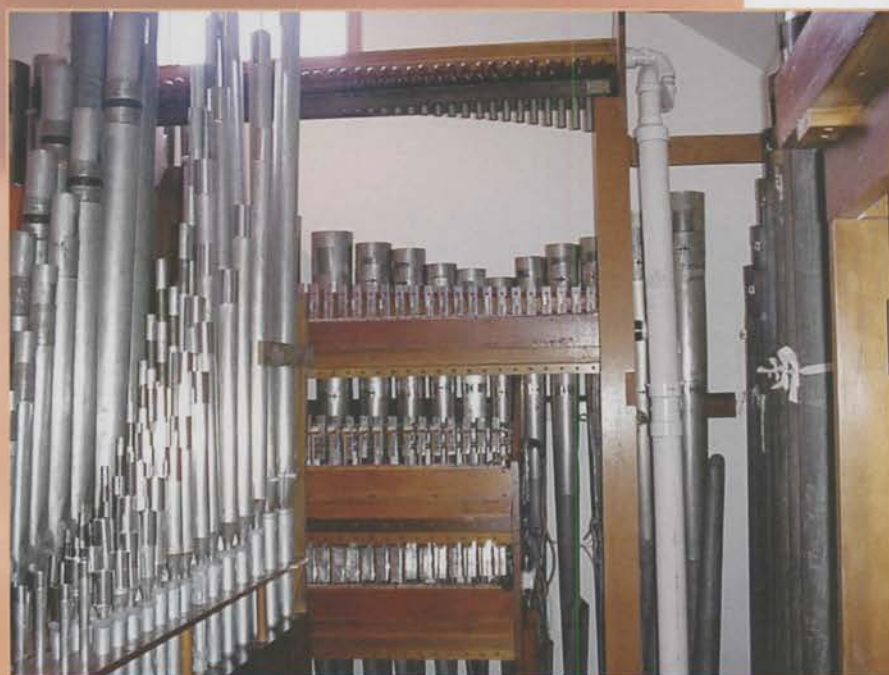
Organ Chamber—Left: Clarinet visible, Straight-ahead: Percussion 'Stack', Bottom: Wurlitzer Chrysoglott, Middle: Glockenspiel, Top: Xylophone. Chimes: (Out of sight) to right.
