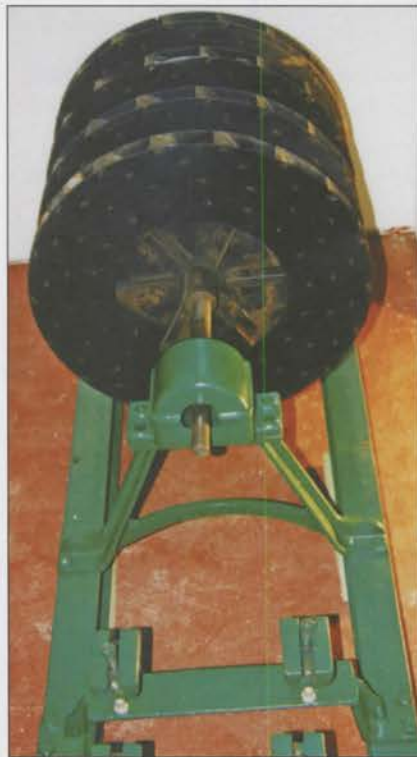
The frame after restoration with the impellers mounted.
