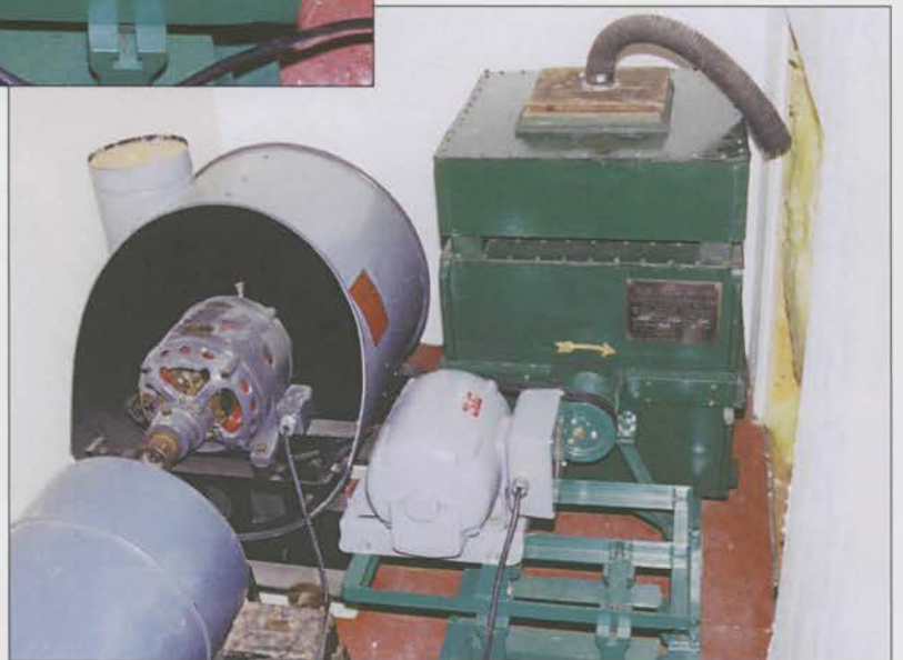
Both the Spencer and Kinetic blower next to each other. These blowers have a similar air flow rating when driven at the same speed.
