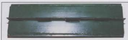
Above: Front of the tool used to spread the top and bottom half of the blower. The sharp edge is driven into the seam and used to spread it apart. Below: Back of the section spreader shows "shiny" bolts used to spread the sections. The other bolts keep the spreader together.
