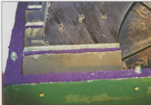
The blower with the top half removed. The tongue that keeps the top and bottom baffles is visible. Notice the "tabs" holding the impeller together.
