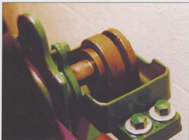
Outboard bearing with cap off. Notice spacer that keeps shaft from damaging bearing when blower slows down.
