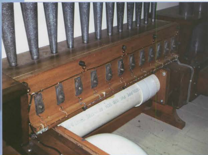
The challenge was to fit the 8' Solo String bass between the 16' Tuba offsets. When no offset chest could be found to fit within our tight parameters, Rick Swanson turned out a beautiful new offset that did.
