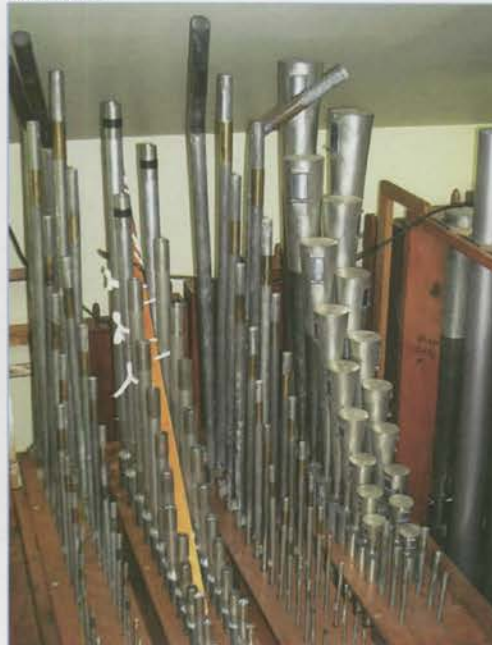
Main chamber shot depicting Wurlitzer Salicional, Kimball Clarinet, Wurlitzer Voix Celeste and Geneva (Organ Supply) French Horn.
