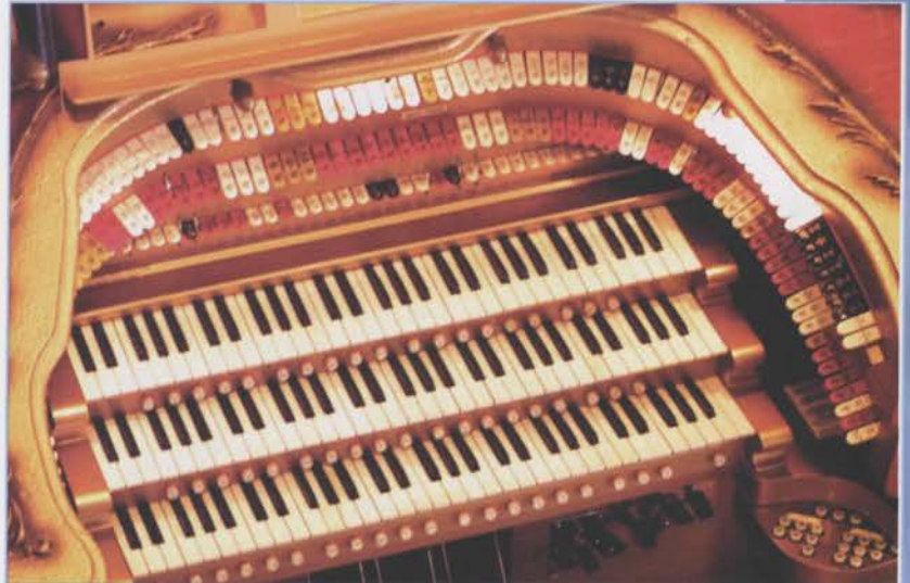
For the stop tablets and identification tags, the type font, abbreviations and most nomenclature was done in Barton style, but their order was rearranged by dynamic level within a given pitch, as used by Wurlitzer. Likewise, piston buttons were engraved in the unique Barton style, but numbered as one would find on a Wurlitzer; the exception being a Divisional Cancel for each keyboard (ala Barton), as well as "Set" and "General Cancel" buttons. In other words, visually, it's a Barton, but ergonomically, it's a Wurlitzer.
