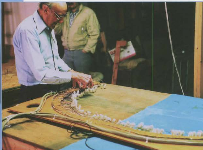
George Gephart wiring plugs for electric stop action magnets.
