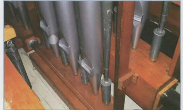
With a ceiling height in both chambers that dramatically reduces from 10' to 6' over a distance of 16' from side to side, we found it necessary to reorient the order of the 8' bass octaves of the Open Diapason and French Horn in order to accommodate it.
