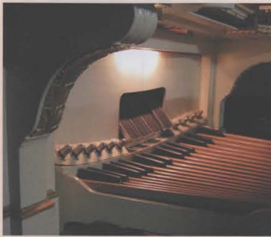
Third swell shoe originally controlled Percussion Chamber and is now unused.
