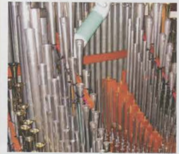
L-R (Solo Chamber front to rear): Orchestral Oboe, Brass Saxophone, Horn Diapason, Quintadena, Oboe Horn, Musette, Solo Tibia, Gamba Celeste, Gamba, Cor Anglais, Brass Trumpet and 16' Horn Diaphone. Gamba 8' across left end of chests.
