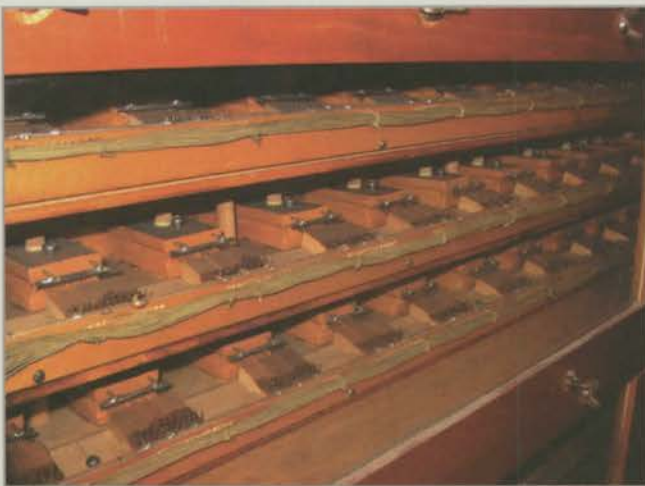
Some of Orpheum's key relays are visible behind glass front of the pressurized case that holds them.
