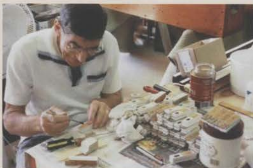
Frank George, one of many volunteers who spent untold hours releathering pneumatics as part of the restoration process.
