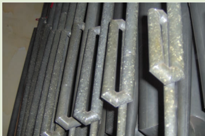
Beautifully made miters of the 16' English Horn. This infamous set of pipes is voiced on 20" wind pressure. Also visible behind are the miters of the 16' Tuba pipes. The 16' Tuba is also voiced on 20" wind.
