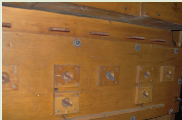
Unique three-stage valve system on the 16' Tibia chest: The single primary valve on the right fires the two secondary actions on the left. These in turn fire the large tertiary pouches under each 16' Tibia pipe toe. Note the two regulating slides between the toes and the tertiary valves.
