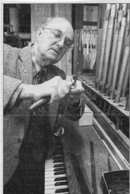
EDWARD STOUT examines an organ pipe. He uses the voice machine (under his left elbow) for testing pipes and making corrections on how they sound. ARIC CRABB — Staff
