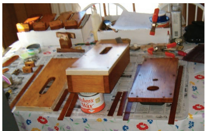
After a thorough cleaning, all wood parts are given a fresh coat of shellac
