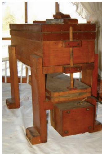
This early #3 Wurlitzer Tremulant (Part Number XA9R) awaits restoration. After many decades, the device has failed completely: it is filthy and all hardware has corroded
