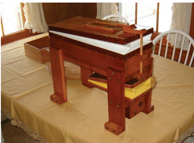
This #3 Tremulant has been completely restored and is ready for another 60 years of service
