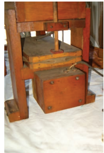
The start/stop motor shows evidence of the gnawing tooth of time: the motor cloth has become stiff and inoperable; all interior leather must be renewed
