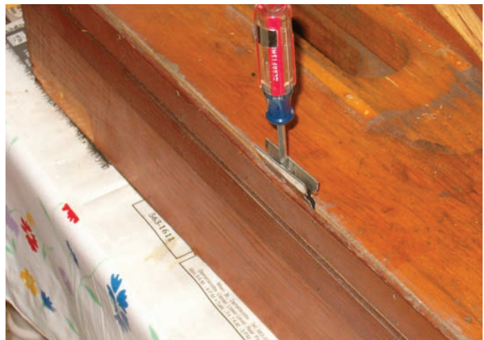
Wurlitzer components were built to be easily restored. During disassembly, all parts are identified and carefully documented with photos and notes. The batten strips of the tremulant head are carefully removed using two single-edge razor blades and a screw driver. Such techniques are used by the careful restorer to avoid scarring and cracking
