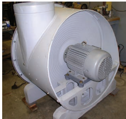
The rebuilt blower (Grahame Davis Collection)
