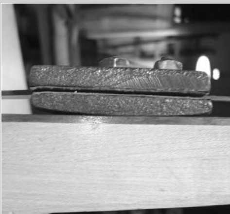
Side view of Barton vibrator mechanism; clearing showing convex shape of inner plate, allowing for near infinite adjustment
