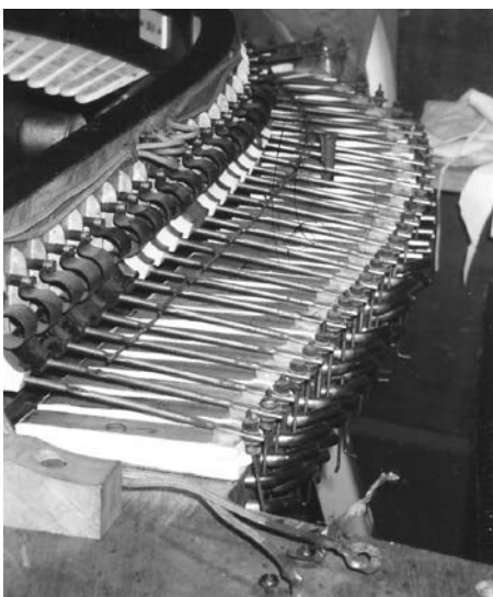
Releathered stopkey pneumatics
