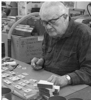
Puget Sound: Russ Evans carefully re-leathers secondary pneumatic motors (Photo by Jo Ann Evans)
