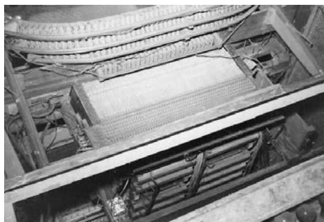
Right: Möller electric stop action magnets
