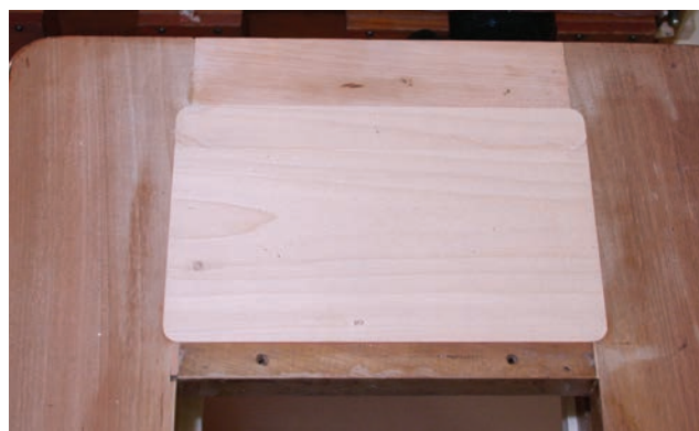
The completed rectangular repair
