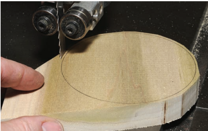
Removing excess wood from the plug blank
