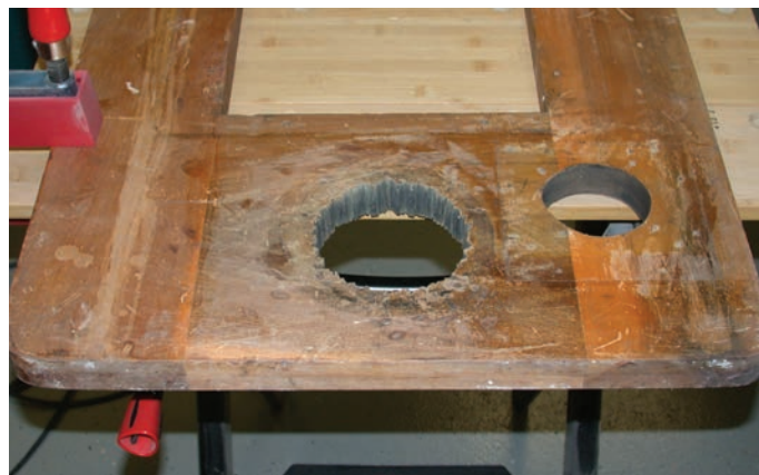
Stripped reservoir back
